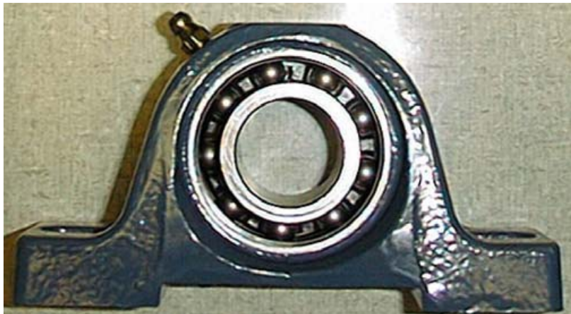
Figure 19. Bearing with Grease Removed
