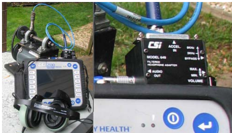
Figure 7. Vibration Analyzer with Headphone Output and Headphone Filtering
