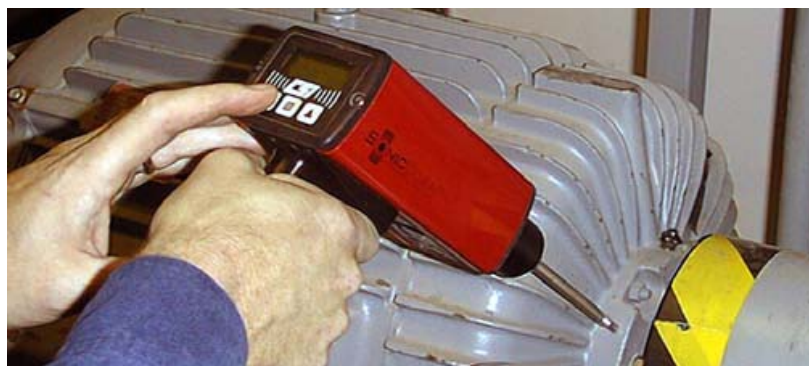
Figure 8. Ultrasonic Analyzer to Measure High-Frequency Lubrication Stress
