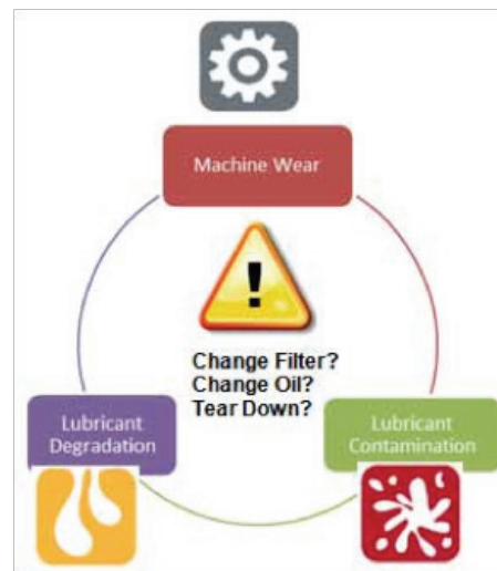
Figure 1: Information provided by in-service oil analysis
