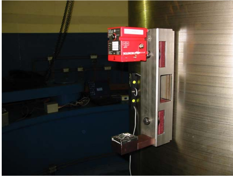
Figure 6. Attaching the PERMAPLUMB to the Hydro Shaft
