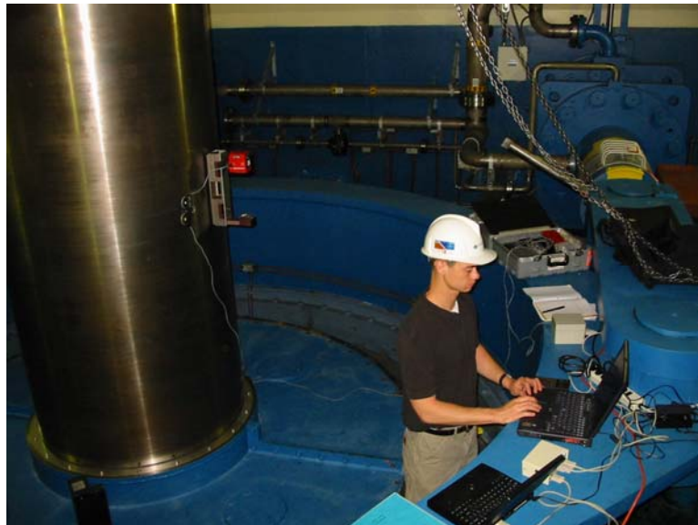
Figure 7. The PERMAPLUMB System Installed on the Hydro Shaft
