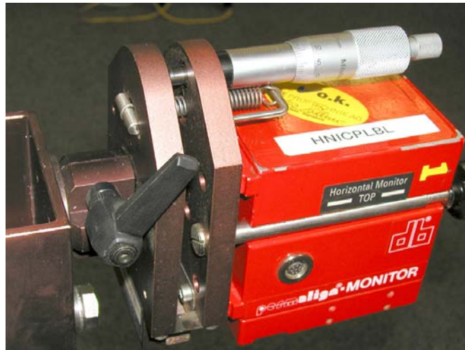
Figure 4. Laser Transducer Mounted upon the Permaplumb Bracket
