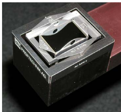
Figure 5. Self-adjusting Mirror Assembly
