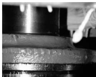
Figure 2a. Inner Cap on Bearing Housing Fitted with Gits Cup
