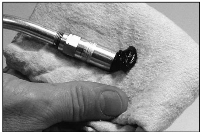
Always make sure the dispensing nozzle of the grease gun is clean before using.
