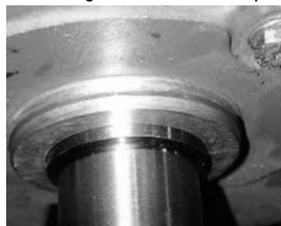
Figure 3. Grease on Labyrinth Seal Outer Diameter and on Inner Cap
