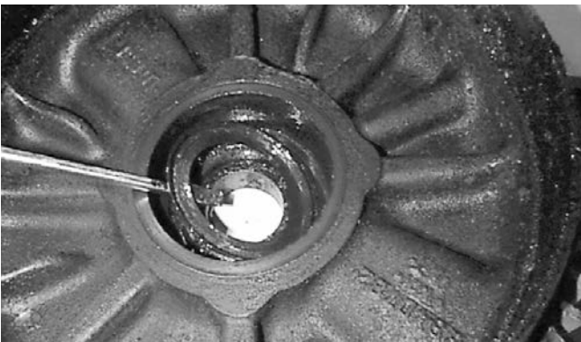
Figure 7. Shield was pressurized by excessive grease which caused a cage failure.
