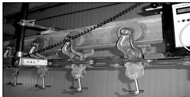
Figure 4. System equipped with automatic paint sprayer marking system designed to mark individual links, which are not found to be within acceptance tolerance limits.
