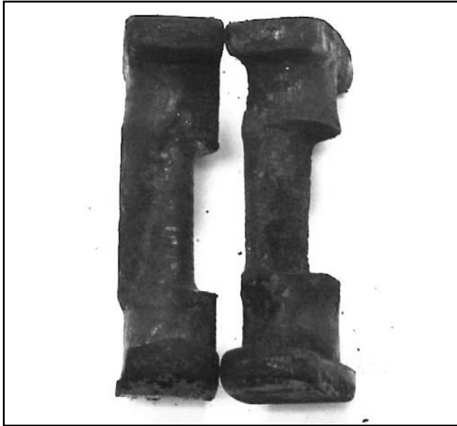
Figure 1. Examples of worn chain pins identified through use of infrared photoelectric chain wear monitoring system.
