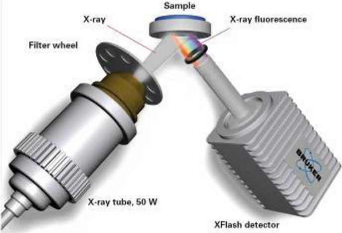
Figure 1 Schematics of ED XRF system
