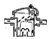
An early warning signal of potential leakage or blow-through in this type of trap will be the rattling sound of the linkage. This indicates linkage looseness that can lead to steam loss.
