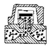
operating in good condition will have a distinctive shut off between discharges, a leaking trap will never shut and will produce a slight hissing sound. Should the disc become worn, a condition referred to as "motor boating" or "machine gunning" can occur. This produces a very rapid rattling sound that closely resembles the above descriptive terms. This condition allows steam to leak through and is a predictor of more severe problems to come.
