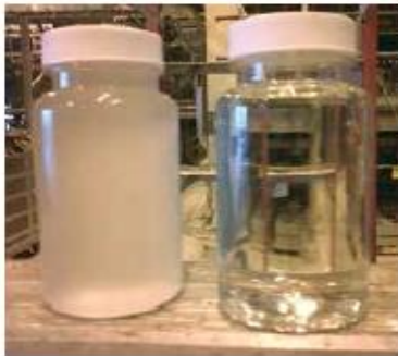
The left beaker pictured is actual hydraulic oil with high levels of moisture and particle contamination at ISO-Cleanliness code 22/21/20. The right beaker shows the same sample after the contaminants were removed at the new ISO-Cleanliness code 18/16/13.
