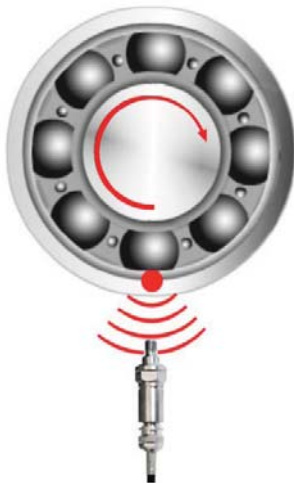
Fig. 10 In a healthy bearing, rollers pass close to the transducer and a high number of low amplitude shocks are emitted from the interface between the roller and the outer race. Each time a roller passes the transducer, the amplitude of the weak shocks increases.
