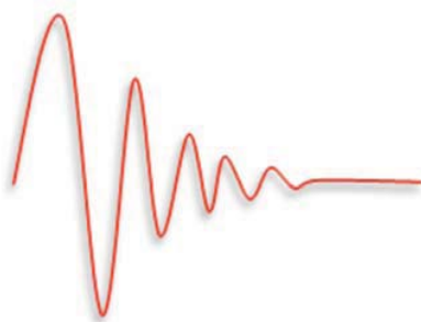
Fig. 4 Typical shock pulse transducer response when hit by a shock pulse. The decay time is short.
