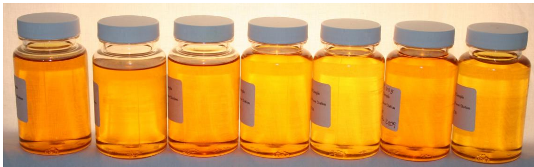
Figure 5. Latest Samples from the 7 GE 7FA Gas Turbines with 48,000 Run Hours
