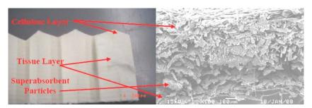
filter media, it readily achieves a capacity of typically 70 times the mass of the entire filter media. That is 70 grams of water per gram of media.
