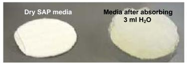
element and that signals the end of the filter's useful life. The photo to the right indicates the physical appearance changes of the SAP media, in this case after absorbing water to the point of a 25 psid (1.7 bar) differential pressure.
