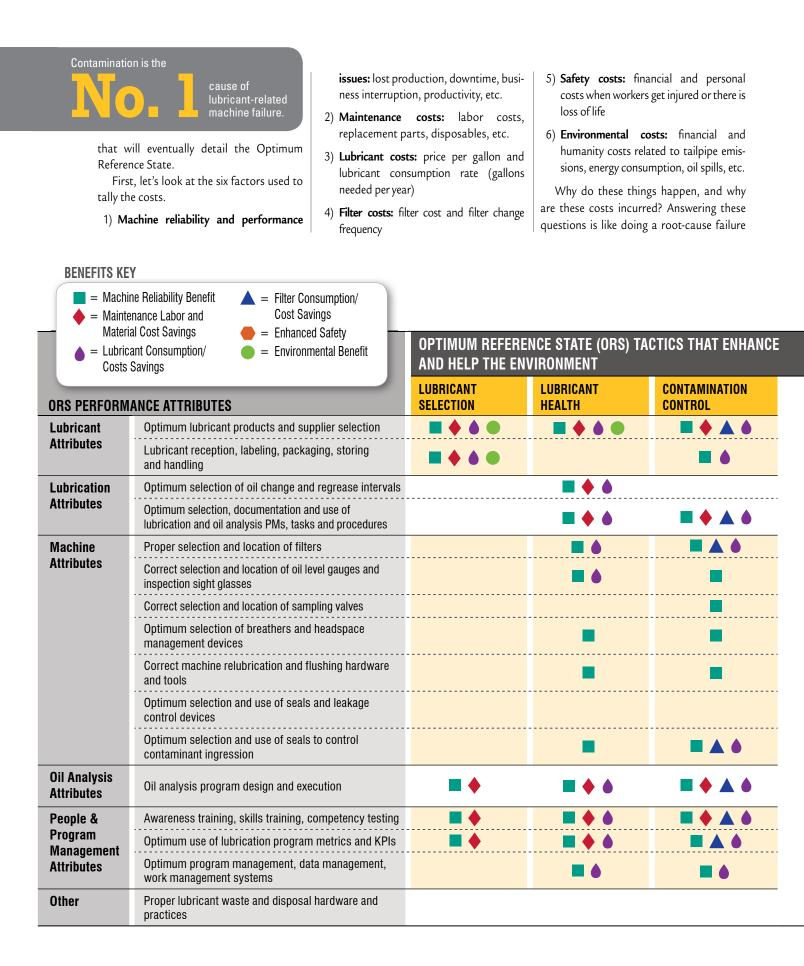
analysis. You have to ask the "repetitive why." The ORS Benefits Grid illustrates how lubrication plays a vital role in reversing or simply reducing the impact in each of the above six cost groups. It also shows the important connection to the Optimum Reference State and a sustained state of cost control and reliability.
